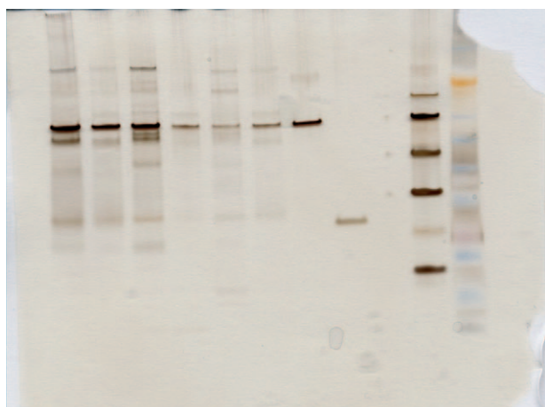
Figure 4. SDS-PAGE of extracts by 4-D10L17PC6 and an avian anti-CRP antibody from human serum. Lanes from left to right: 1) anti-CRP in human serum, 2) anti-CRP in CRP-free serum, 3) 4D10L17PC6 in human serum, 4) 4D10L17 in CRP-free serum, 5) blank, PS beads in human serum, 6) blank, PS beads in CRP-free serum, 7) HSA, 8) CRP, 9), 10) standard proteins (97, 66, 40, 30, 20.1, and 14.4 kDa), 11) prestained standard.
